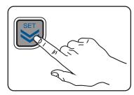
if a selection is not made after 15 seconds, the last value displayed will be confirmed automatically and the chamber temperature display is restored.
